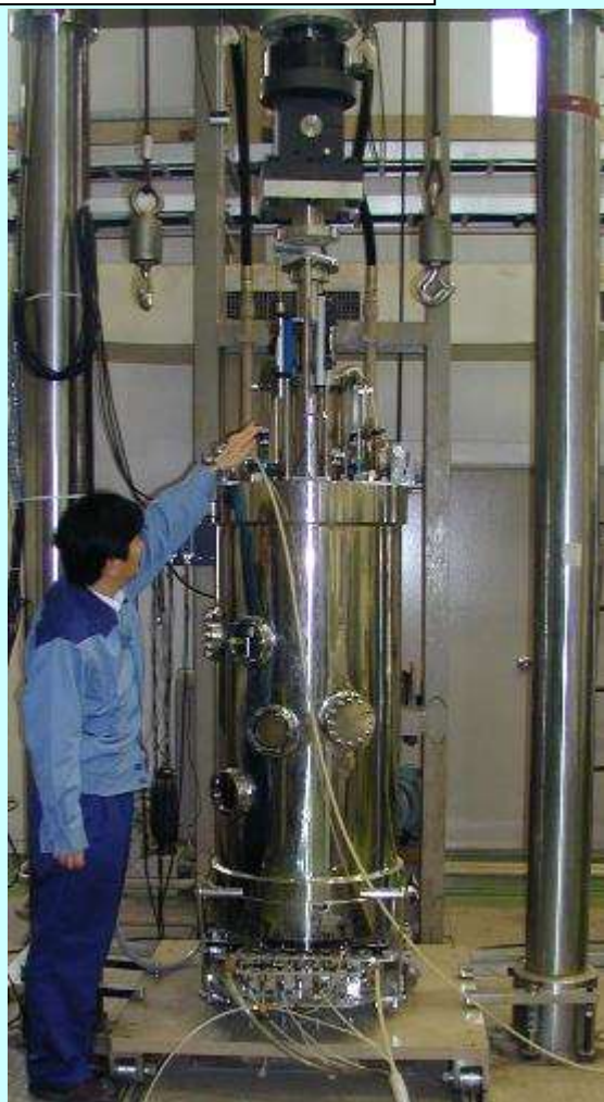
Large dynamic triaxial compression test
