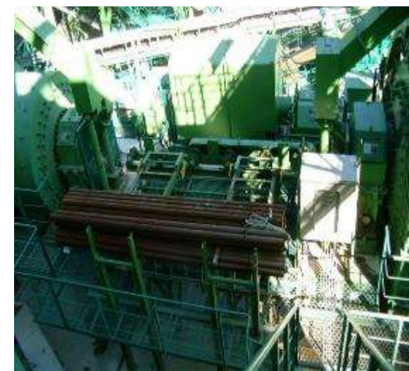
Sand manufacturing facility (Rod mill)
