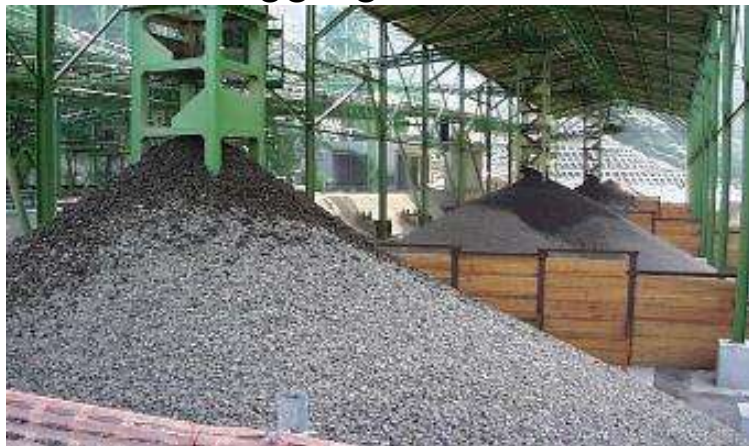
Stockpile for manufactured coarse aggregate
