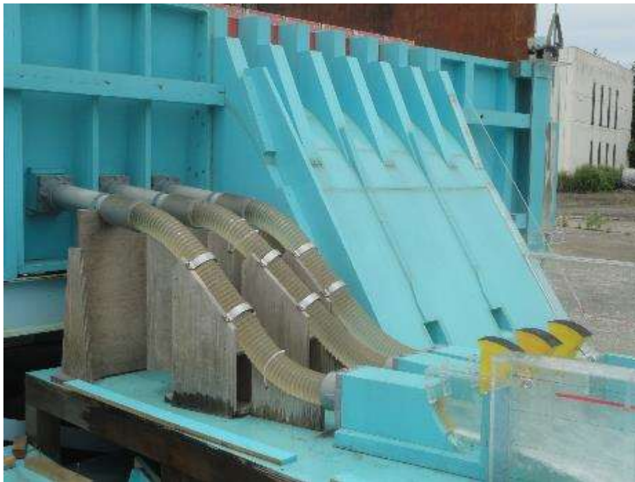
Full model spillways (Sameura Dam scale: 1/62.5)
