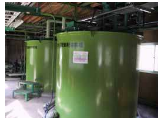
Polymer coagulant dissolution tank
