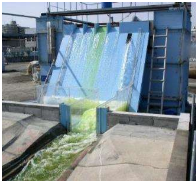
Model test of a spillway of Oyama Dam (Scale:1/40)
