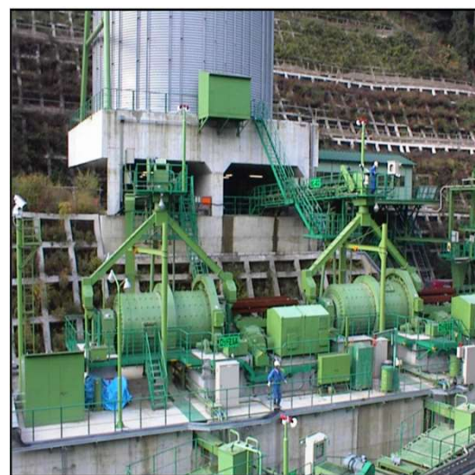
Sand manufacturing facility (Rod mill)
