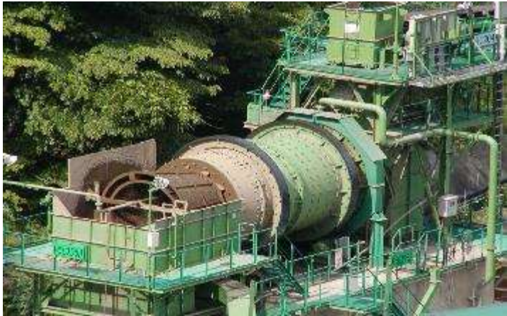
Aggregate washing facility (Drum scrubber)
